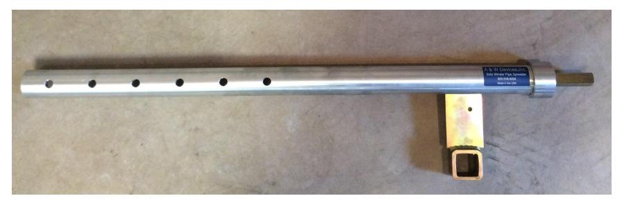
The body of the Side Winder Pipe Spreader is an Aluminum tube. There is an Inner Tube Attachment with an eye for the Screw Assembly. On the end of the tube is where the Outer Tube Attachment slides and is secured at the correct length.
