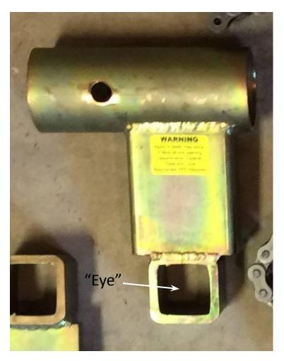
The outer Tube Attachment has a hole on the top tube section to secure the piece to the Tube. The lower portion of the attachment has the "Eye" which is where the Chain/Screw Assembly is threaded. Attach Chain/Screw Assembly to pipe.
